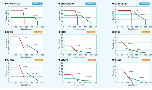
\* Maximum operating speed may drop when an external force is applied or the support guide sliding resistance is large.
