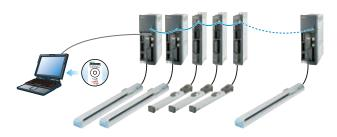
Connecting two or more TS series controllers and drivers in a daisy chain allows editing data on any one unit from a PC.
