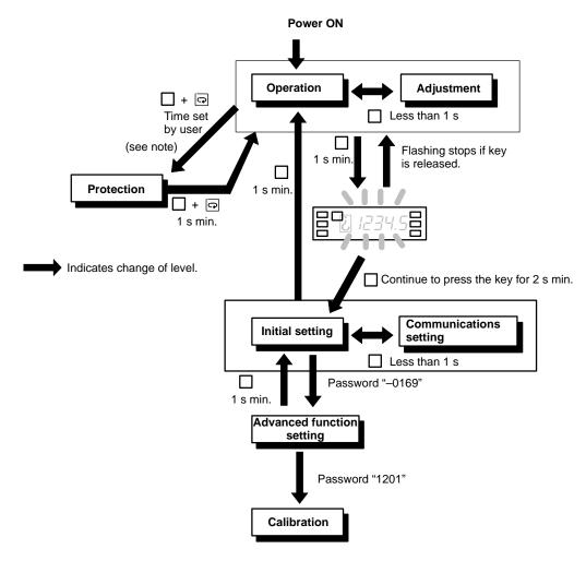
Note: The move to protection level time can be set in the advanced function setting level.
