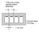
Note: The space between each relay required for heat radiation may vary with operating conditions. Contact your OMRON representative for details.
