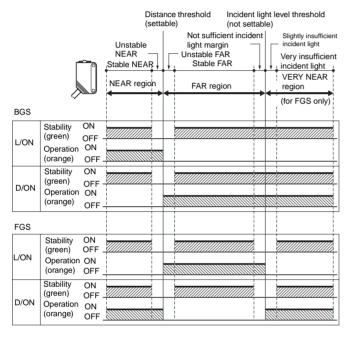
**Note:** 1. If the stability indicator is lit, the detection/no detection status is stable within the rated ambient operating temperature (-25 to 55°C).
