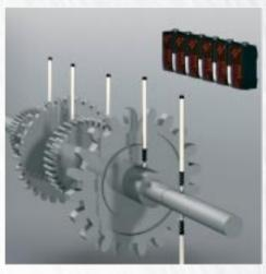
Measuring warp and inclination Integrated calculation functions can be used for P-P or A-B calculation.
