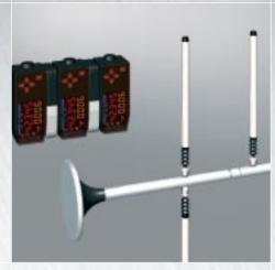
Diameter and eccentricity measurement Measuring the diameter and eccentricity of valves and shafts with a high resolution of 0.1µm can be performed without any influence from surface conditions.
