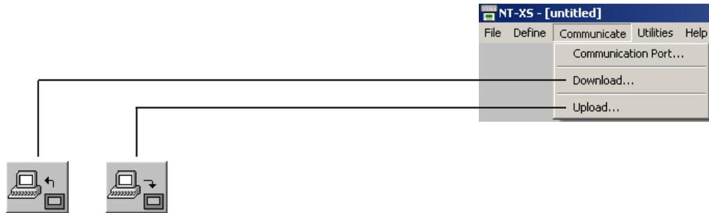
*Communication Port* - Sets COM port for communicating with NTXS .
