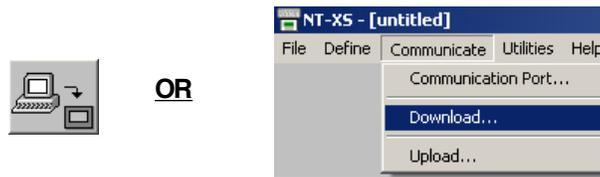
In the download dialog box, check '**Application**' radio-button. Press '**OK**' button to download application to NTXS unit. Following window will be presented for NT2S models.
