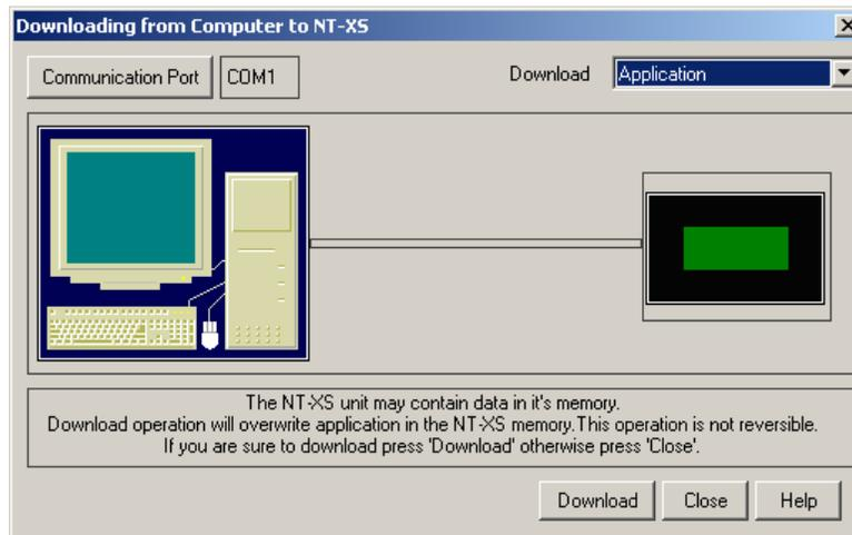
After downloading the application also download the firmware by using the same method as described above but then selecting 'Firmware' instead of 'Application'. This completes the configuration of the unit. Now application will be executed.
