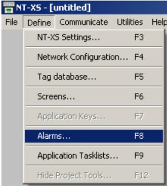
To add alarms, click **ADD** button. Select Tag to be monitored. Select the Alarm group. For first 16 alarms the group is 01, for next 16 alarms group is 02. Alarm number indicates the bit number in the specified tag. Alarm text should be added. Alarm Text is displayed in the alarm window when the alarm is triggered.
