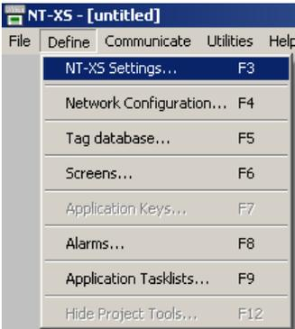
In NTXS Settings dialog box, printer port settings, Max characters per screen for serial printing for NT2S. For NT3S select number of languages. Press **OK** to accept the selections made.
