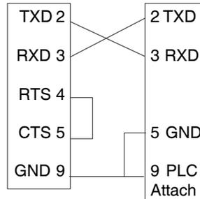
**Pin Configuration for communication cable between XtraDrive and NT3S:**
