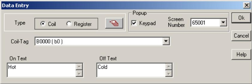
For NT3S models, either a pop-up keypad should be enabled or a numeric keypad should be placed on the screen. A pop-up screen pops up only when user selects a data entry object. This screen generally has a numeric keypad.
